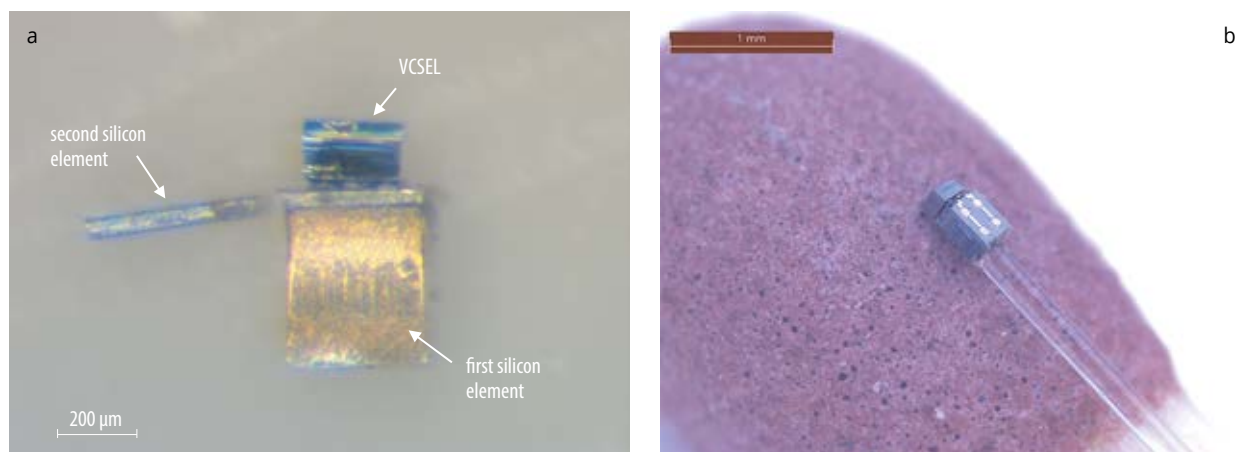
Fig. 2 (a) Side view of an ODLM F2R interposer with assembled VCSEL, released from the Si frame. The two silicon elements are connected by flexible interconnects. (b) An assembled ODLM, with the VCSEL and an inserted 125 \mu\text{m} diameter optical fiber, placed on a match head. The optical fiber was fixed with biocompatible glue.
