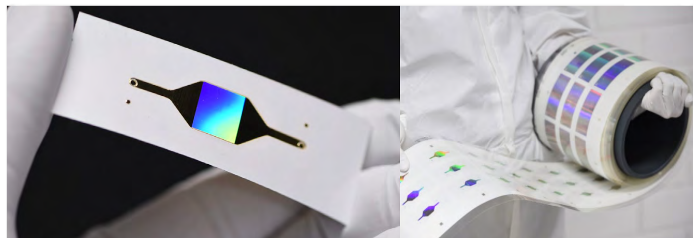
Sensor chips with plasmonic surface and integrated microfluidics
