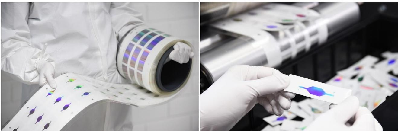
Figure 5. Left: Roll of complete sensors. Right: Sensor singulated from the roll by rotary kiss cut process.
