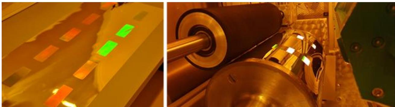
Figure 12. Manually fabricated polymer shim after fabrication (left) and mounted in the R2R pilot line (right).
