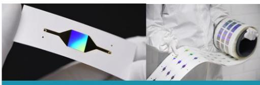
Sensor chips with plasmonic surface and integrated microfluidics
